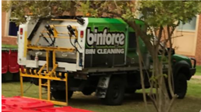
Figure 4-2 On-site bin wash system for rear-lift trucks on back of ute. Source: http://binforce.com.au/
